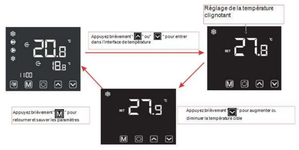
Comments: In the temperature setting interface, if you briefly press , the system will return to the main display and no changes will be saved. When the temperature appears on the display after you set the value you want, wait 5 seconds and the temperature displayed will be saved as the set temperature. The system will automatically store the user setting and return to the main interface.
